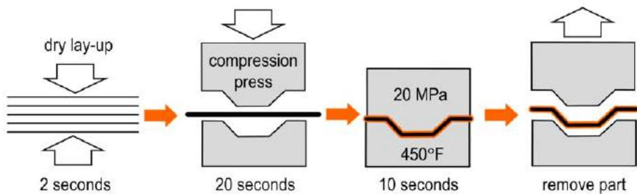
*Figure 3. High speed consolidation and molding for Mallinda's malleable materials*
