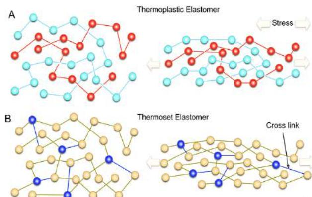
Figure 1. Thermoplastics vs. Thermosets
