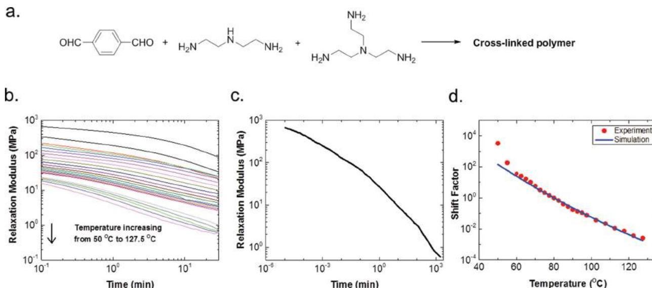
**Figure 1.** Polymer synthesis and stress-relaxation studies. a) Synthesis of crosslinked polyimine. b) Stress relaxation curves at various temperatures over a time period of 30 min. This data was used for the temperature-time superposition calculations. c) Temperature-time superposition master curve derived from data in Figure 1b. d) Shift factor vs. temperature plot for temperature-time superposition experiment. The blue line is derived from 80 °C reference temperature data from Figure 1c.
